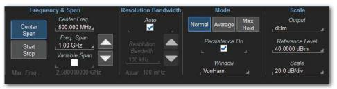
Spectrum analyzer style controls simplify waveform analysis in the frequency domain.
